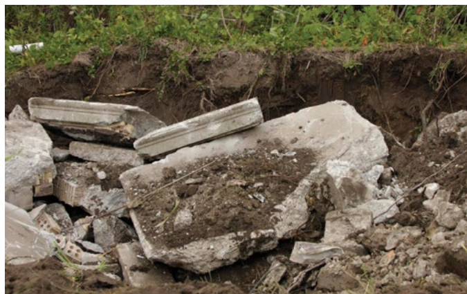
Figure 8. Salvaged materials, such as used concrete slabs and construction blocks, can be used for hibernaculum construction. Left: © G. Beck; Right: © WEIS
